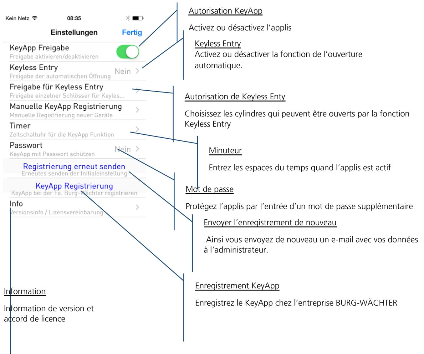
The screenshot shows the 'Einstellungen' (Settings) screen for the KeyApp. The status bar at the top indicates 'Kein Netz' (No network), the time '08:35', and battery level. The settings list includes:
